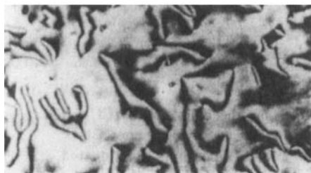
Figure 5. The optical microscopic texture observed for the BB-5 smectic phase in a homeotropic alignment.
